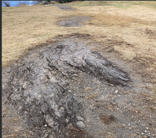
In-place interlayered micaceous biotite gneiss and schist exposed under the Duke power lines. Note the cross-cutting quartz veins and the foliation of the rock, dipping or sloping to the right, or northwest.
