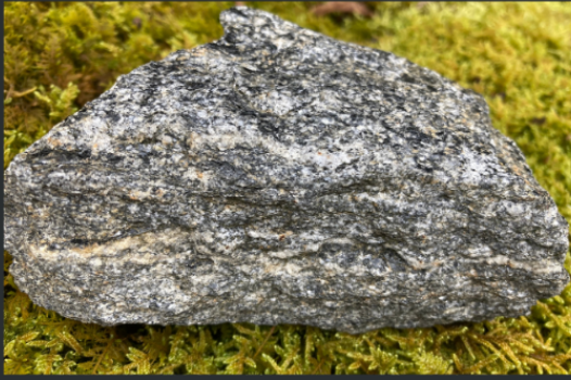
Hand specimen" (about 4" long) of micaceous gneiss from the Graywacke-Schist member of the Tallulah Falls Formation. Gray and white are quartz and feldspar; black is biotite mica. Note the right to left banding or foliation planes of the minerals, typical of metamorphic gneiss and schist.
